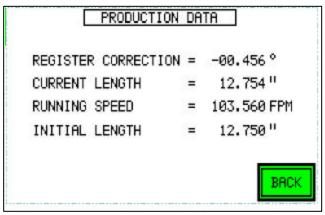
Register Correction shows the size of the correction of your repeat length measured in degrees. A negative number represents a retard correction.
