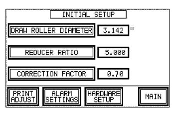
Press "DRAW ROLLER DIAMETER." The diameter of the feed roller must be accurately measured and entered into the program.
