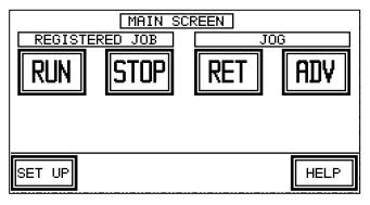
Press "SET-UP" to access the Set-Up Screen.
