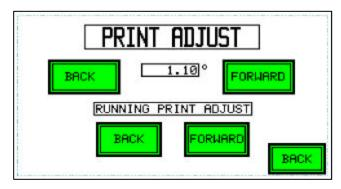
To reposition the actual cut position of the web, press "Forward or Back."
