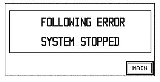
During machine jams, a following error may exist when the servomotor is two rotations out of position with the knife encoder. The following error will stop the Servo System.
