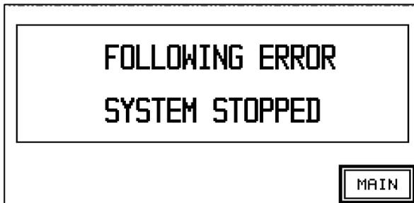
During machine jams, a following error may exist when the servomotor is two rotations out of position with the knife encoder. The following error will stop the Servo System.
