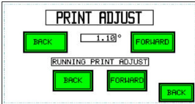
To reposition the actual cut position of the web, press "Forward or Back."
