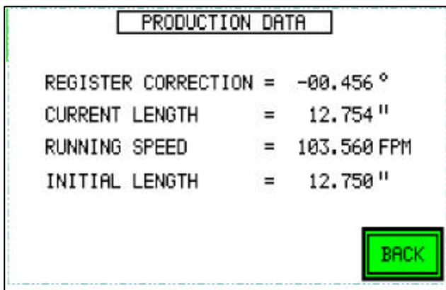
Register Correction shows the size of the correction of your repeat length measured in degrees. A negative number represents a retard correction.
