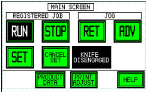
On labelers, an existing limit switch informs the EMP Servo System when the knife is disengaged. At this point the labeler is not ready to feed labels.
