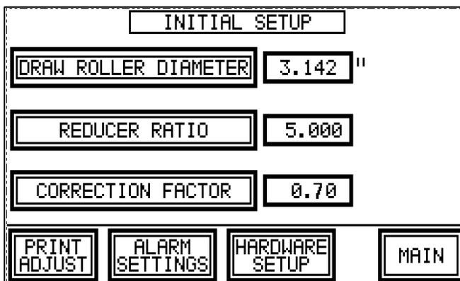
Press "DRAW ROLLER DIAMETER." The diameter of the feed roller must be accurately measured and entered into the program.
