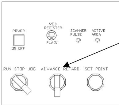
The position of the Cut can be adjusted on an operating machine using the ADVANCE RETARD switch.
