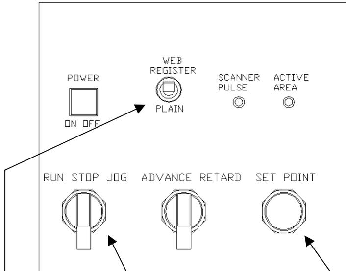
Put the "RUN STOP JOG" switch in STOP.
